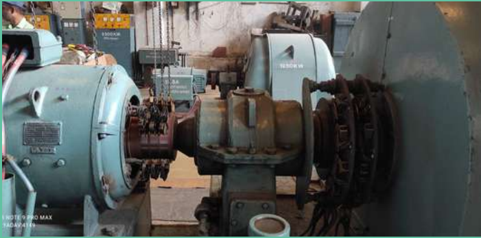
Turbine coupled with DC Generator
